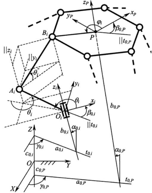
Fig. 2. Geometry of the  $i$ -th leg of the PM
