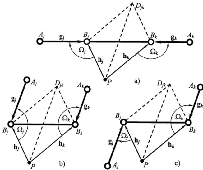
Fig. 4. Layouts of  $j$ -th and  $k$ -th passive links of PM in a plane of a mobile platform
