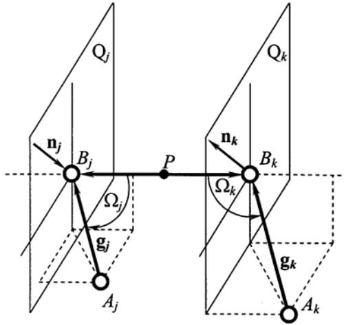
Fig. 3. Spatial layouts of vectors of  $j$ -th and  $k$ -th lines of a Jacobian  $\mathbf{A}$  in a case when  $\mathbf{n}_j \neq \mathbf{0}$ ,  $\mathbf{n}_k \neq \mathbf{0}$ , and  $\mathbf{h}_j \parallel \mathbf{h}_k$
