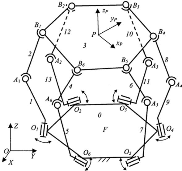
Fig. 1. Six-legged PM with 6 DOF
