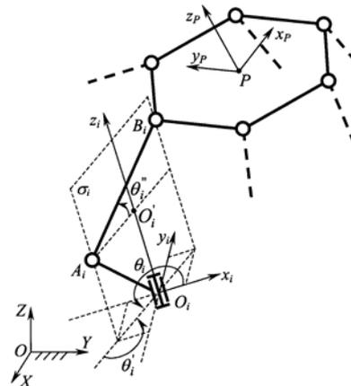
Fig. 3. The first type of singularity of the PM
