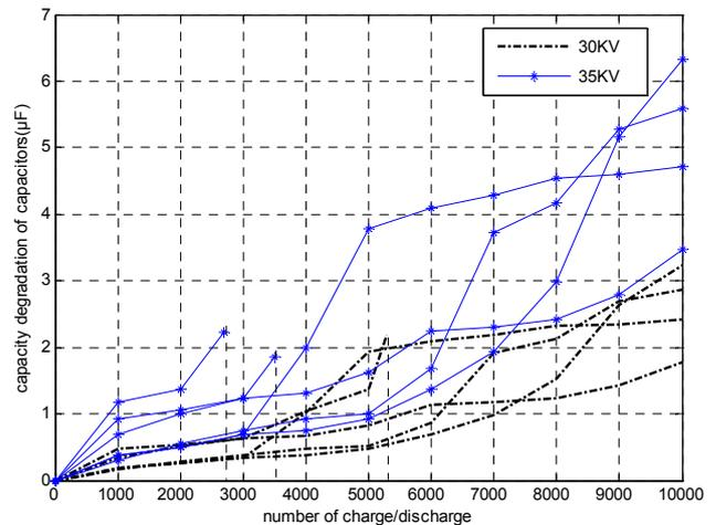
Fig. 1 the capacity accelerated degradation data of capacitors
