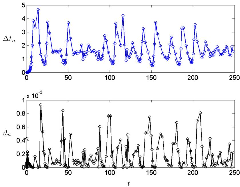
Figure 5: Local linearity control. Top frame: step selection. Bottom frame: monitor function  $\vartheta_n$ .
