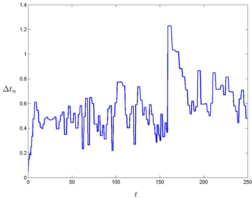
Figure 2: Step-sizes used by ODE45 in solving (3).
