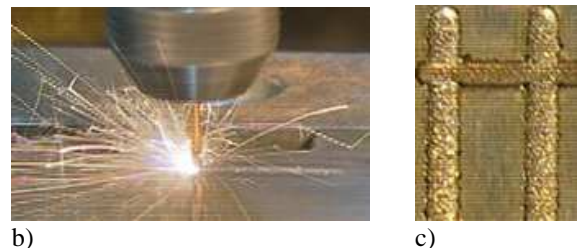
Figure 5: Scheme of the machining process kinematics (a) and machining process (b) and machined surface (c)
