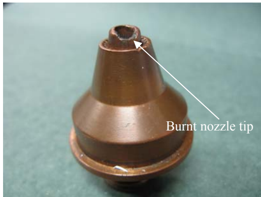
Figure 8: Burnt nozzle due to reflected heat at 3 kW laser power.
