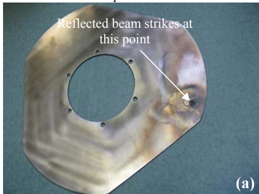
Figure 8: Burnt nozzle due to reflected heat at 3 kW laser power.
