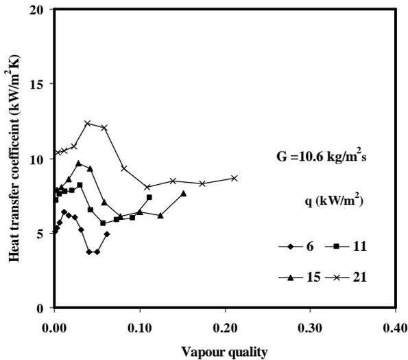
Fig 4: Heat transfer coefficient against vapor quality for mass flux of 10.6kg/m<sup>2</sup>s
