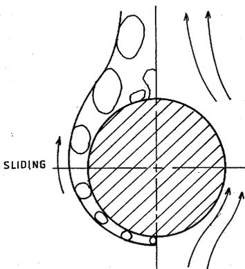
Fig 2: Sliding bubbles on a horizontal tube, Cornwell and Schuler [14]
