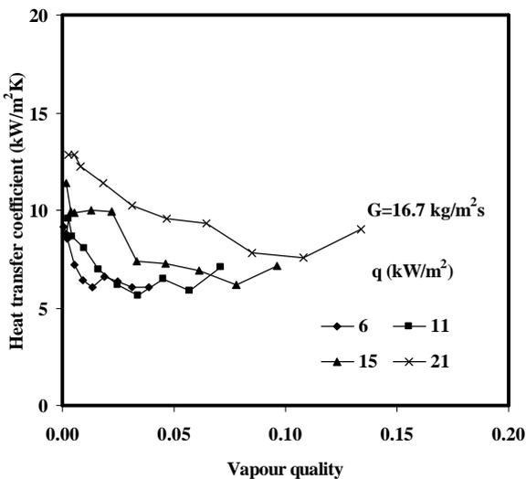
Figure 5: Heat transfer coefficient against vapor quality for mass flux of 16.7 kg/m<sup>2</sup>s
