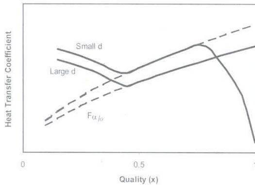
Figure 1 heat transfer coefficient with quality for tube bundles with large and small diameter tubes, Cornwell, Kew et al [10]
