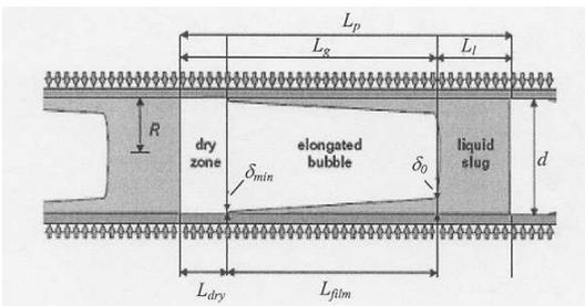
Fig 3; Diagram illustrating the three zone model of Thome, Dupont et al [21]
