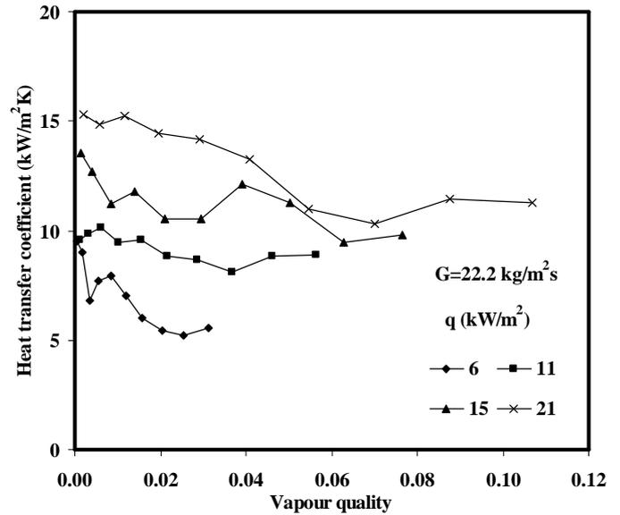
Figure 6: Heat transfer coefficient against vapor quality for mass flux of 22.7 kg/m<sup>2</sup>s
