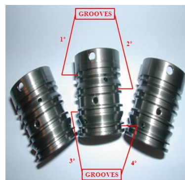
Figure 5 – Grooves of sleeve for pinion & valve assembly of steering mechanism.
