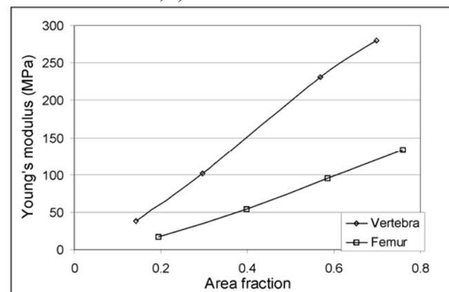
Fig. 4. Apparent Young's modulus as a function of area fraction occupied by trabeculae for vertebra and femur.
