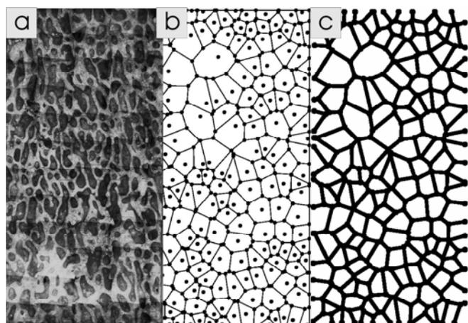
Fig. 1. a) Original microstructure obtained by stitching together several optical microscopy image. b) Forming points and the corresponding Voronoi partition of a part of the zone of interest. c) Reconstructed, synthetic microstructure.
