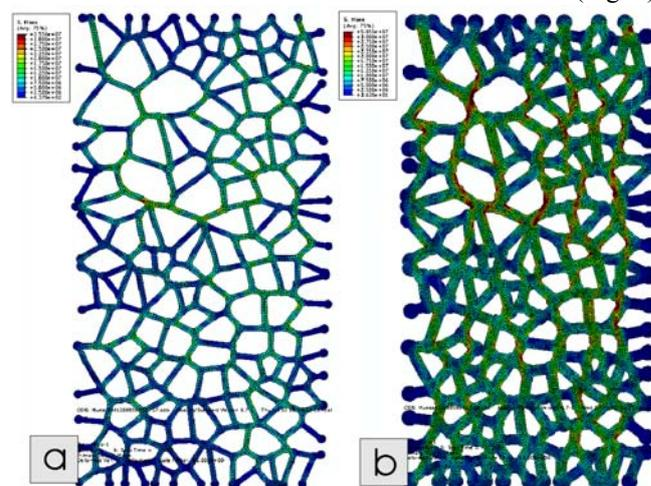
Fig. 2. Stress distribution in a synthetic microstructure based on the forming points obtained from a micrograph of trabecular bone from bovine femur. a) Corresponds to an area fraction of 40%, b) to 76%.
