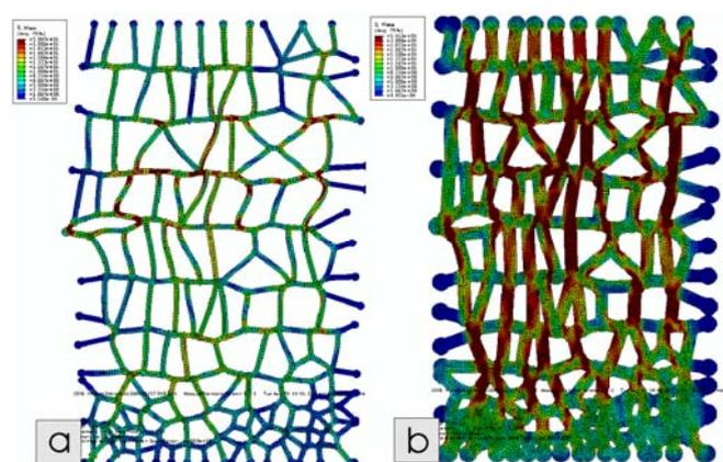
Fig. 3. Stress distribution in a synthetic microstructure based on the forming points obtained from a micrograph of trabecular bone from bovine vertebra. a) Corresponds to an area fraction of 30%, b) to 70%.
