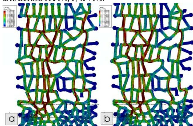
Fig. 5. Stress fields in the synthetic structures based on vertebral tissue, with 4 and 8% loss of trabeculae by number. The random assignment of the eliminated trabeculae converts
