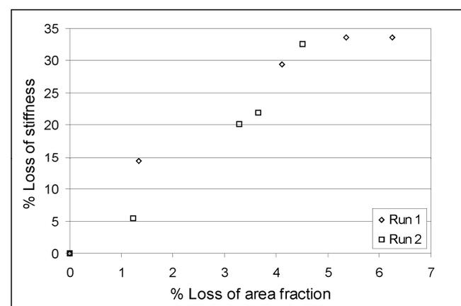
Fig. 6. Graphic representing the loss of stiffness as a function of the loss of area fraction in the synthetic structure for vertebral cancellous bone. Trabeculae were removed in steps
