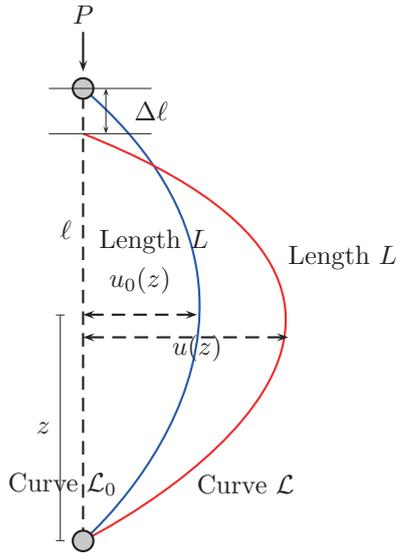
Figure 2: The buckling of an initially curved rod.
