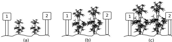
Figure 4. The different stages of the plant growth have different effects on signal attenuation: (a) no attenuation since plants are below the antennas Line-of-Sight; (b) the plants start to cover the path between antennas and its effect starts to be noticed; (c) plants totally cover the path between antennas causing a maximum attenuation.
