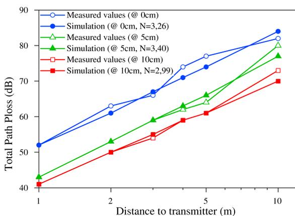
Figure 7. Comparison between the measured and the simulated values for the free-space attenuation, for various distances to the transmitter, at different distances to the ground.
