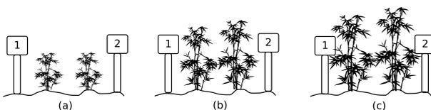
Figure 4. The different stages of the plant growth have different effects on signal attenuation: (a) no attenuation since plants are below the antennas Line-of-Sight; (b) the plants start to cover the path between antennas and its effect starts to be noticed; (c) plants totally cover the path between antennas causing a maximum attenuation.
