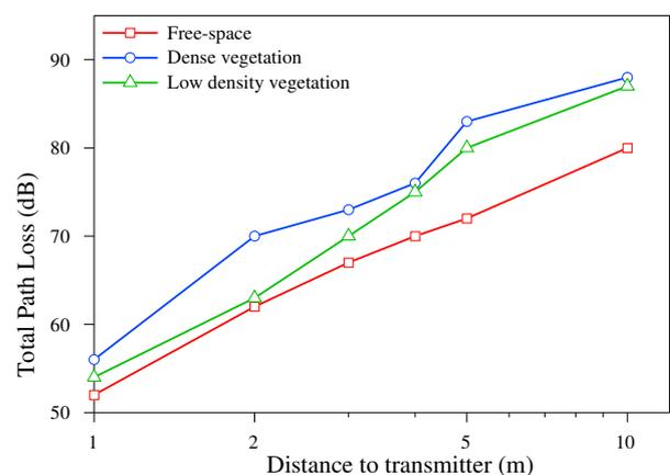
Figure 5. Comparison between the different attenuation values, measured at various distances to the transmitter with different propagation medium: free-air, dense grass/weeds and low-density vegetation at ground level.
