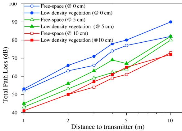
Figure 6. Comparison between the different attenuation values, measured at various distances to the transmitter, at different distances to the ground, in free-space and in low-density vegetation.
