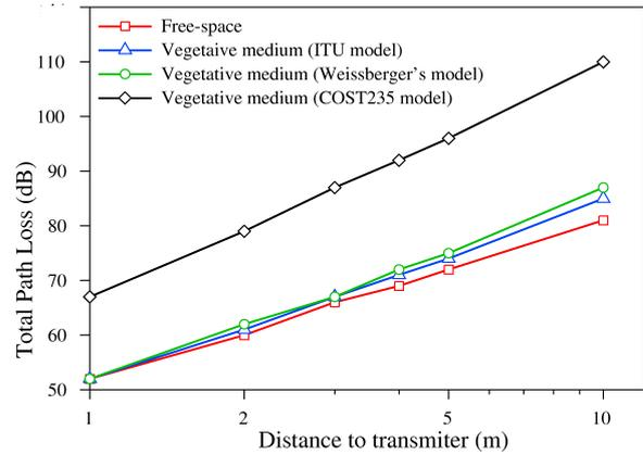
Figure 2. Simulation of electromagnetic waves attenuation in free-space and in vegetative mediums, using the ITU, the Weissberger and COST235 models.
