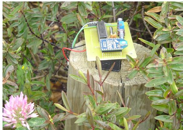
Figure 3. Prototype based on a 8-bit microcontroller and XBee module.
