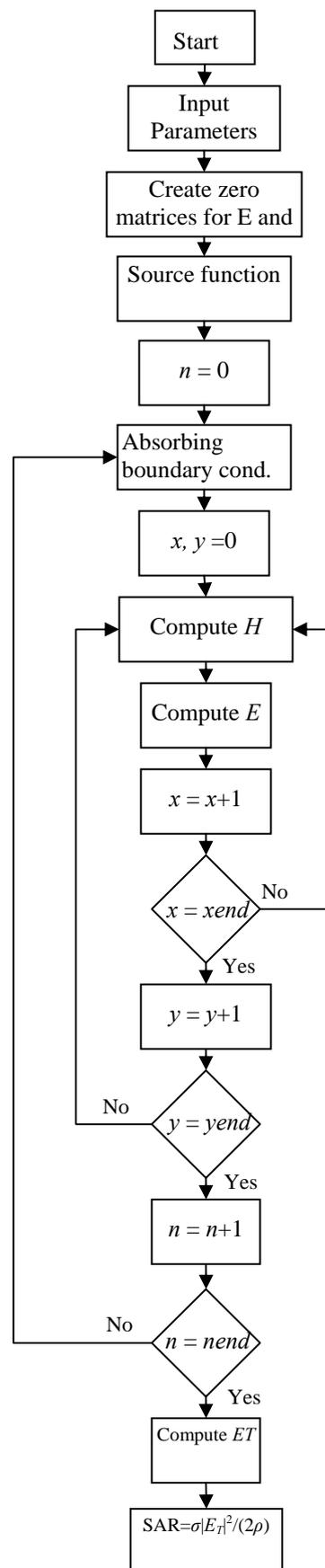
Figure 2. Flow diagram for developed program
