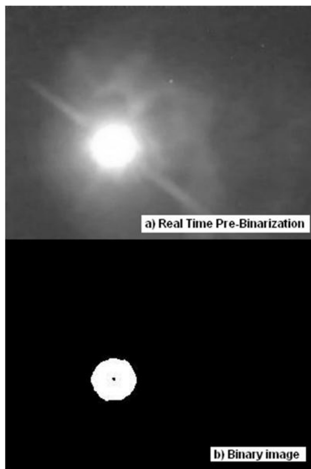
Fig.1. Processing of one frame. a) Result of real time Pre-Binarization. b) Calculus of the coordinates of the centroid.
