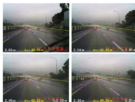
Fig. 14. The results of preceding vehicle detection in heavy rainy day in an image sequence.
