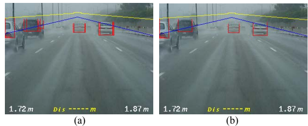
Fig. 8. The result of deleting overlapping candidates. (a) The detected candidates. (b) The reserved candidates after deleting overlapping candidates.
