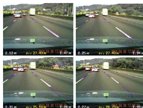
Fig. 11. The results of preceding vehicle detection in sunny day in an image sequence.
