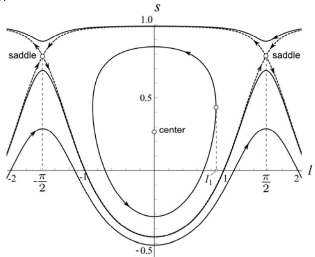
Fig. 2. Phase trajectory for the oblate gyrostat:  $I_2 = 2.1 \text{ kg m}^2$ ,  $I_3 = 1.6 \text{ kg m}^2$ ,  $I_p = 2.5 \text{ kg m}^2$ ,  $d = -0.15$ , ( $s_c = 0.267, s_s = 0.788$ )
