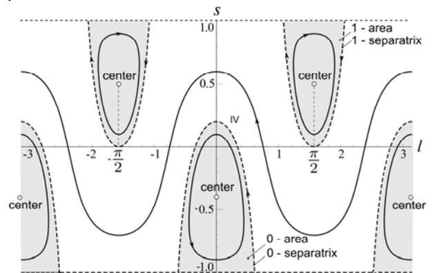
Fig. 4. Phase trajectory for the intermediate gyrostat:  $I_2 = 2.0 \text{ kg m}^2$ ,
