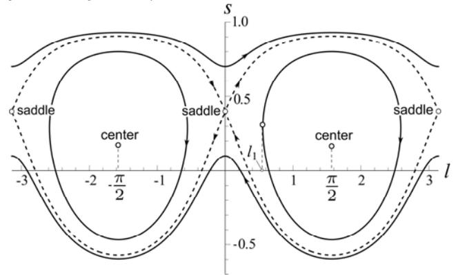
Fig. 3. Phase trajectory for the prolate gyrostat:  $I_2 = 2.0 \text{ kg m}^2$ ,  $I_3 = 1.6 \text{ kg m}^2$ ,  $I_p = 1.4 \text{ kg m}^2$ ,  $d = 0.05$  ( $s_s = 0.4, s_c = 0.167$ ).
