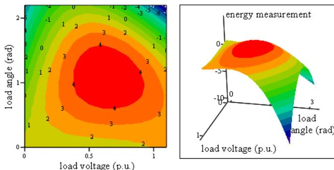
Fig. 6. System's stored energy for  $\delta_m=1.6$  (a) Two-dimensional representation (b) Three-dimensional representation.
