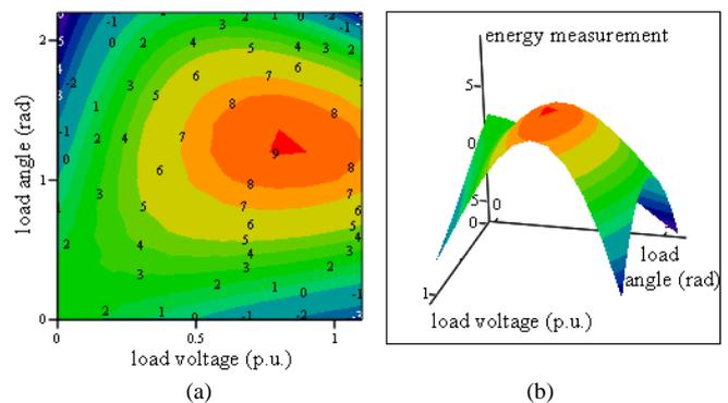
Fig. 2. System's stored energy for  $\delta_m=0$  (a) Two-dimensional representation (b) Three-dimensional representation.
