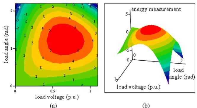
Fig. 5. System's stored energy for  $\delta_m=1.2$  (a) Two-dimensional representation (b) Three-dimensional representation.
