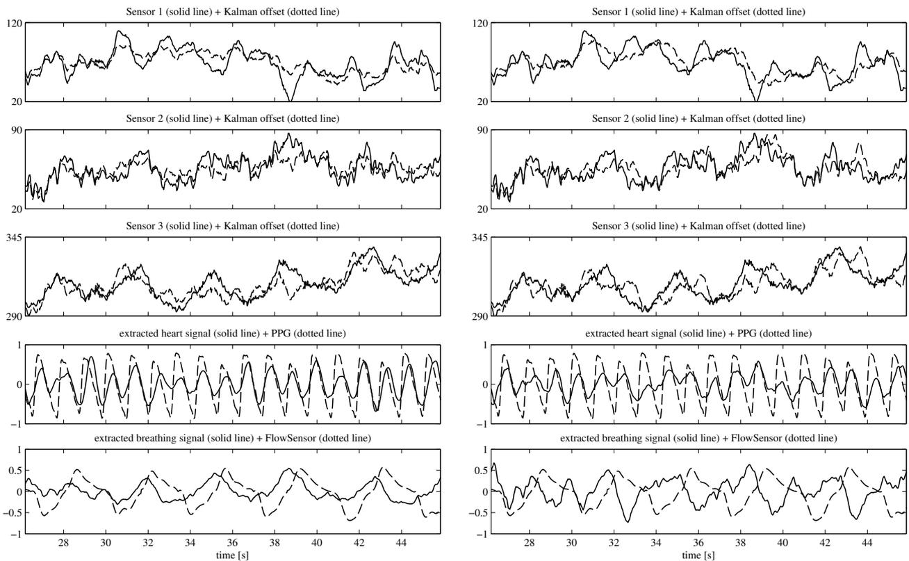
(a) Good breathing and heart frequency estimations (with  $f_s = 0.26 \text{ Hz}$  and  $f_f = 0.9 \text{ Hz}$ ).
