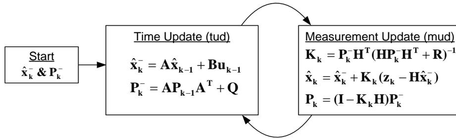
Fig. 2. Schematic way of iterative Kalman Filter parameter calculation ([2][8][9])
