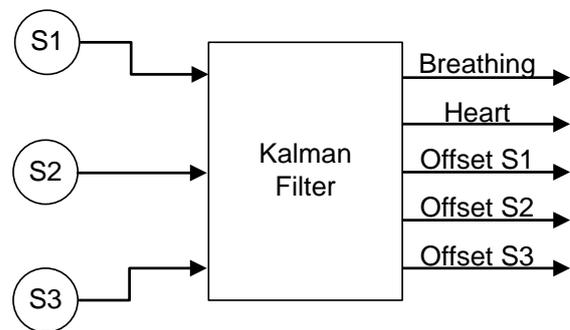
Fig. 1. Kalman Filter Sensor Fusion (Sensors: S1 to S3) and Vital Signs Extraction
