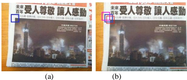
Fig. 7. An example of corner point tracking. (a) front image frame and a blue square R centered at a corner point (b) current image frame and a red square R' centered at the corner point was detected using mean shift tracking algorithm..
