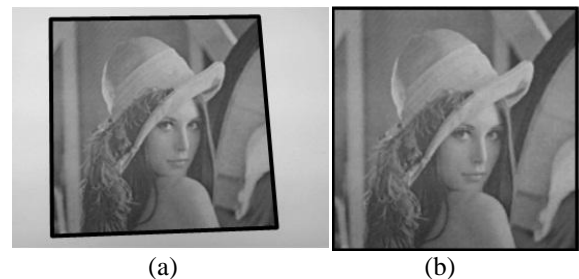
Fig. 6. An example of four-point transformation. (a) the image taken by a webcam (b) the calibrated image using the four-point transform.
