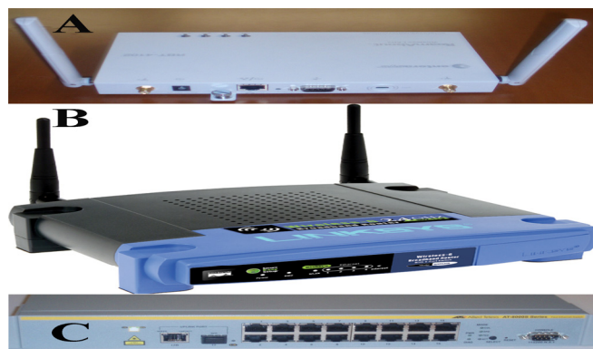
Fig. 1- Access point (A) [11], Wireless router (B) [13] and switch (C) [12].
