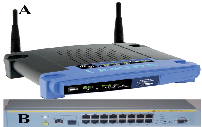
Fig. 1- Wireless router (A) [13] and switch (B) [15].
