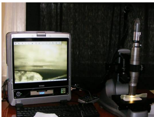
Fig.3 Keyence digital microscope connected to PC
