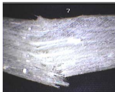
Fig.13 Sample 7, bending, 5x
