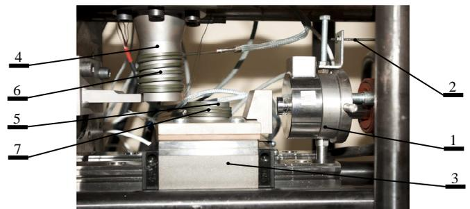
Fig. 5 Shearing assembly of the test facility 1 – shear force sensor, 2 – cylinder position sensor, 3 – ball bearing slides, 4 – fixed tube, 5 – moving tube, 6 – upper heating coil, 7 – lower heating coil.
