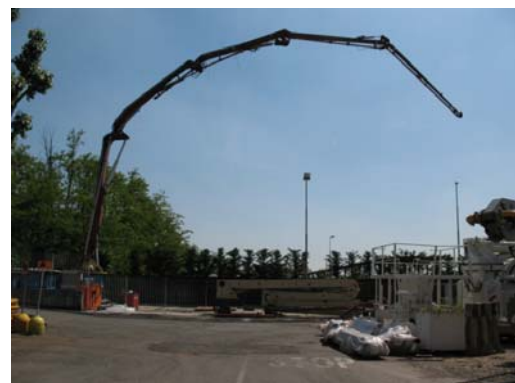
Fig. 4. The boom test rig
