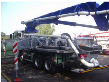
Fig. 2. The pumping group unit bolted on the truck
