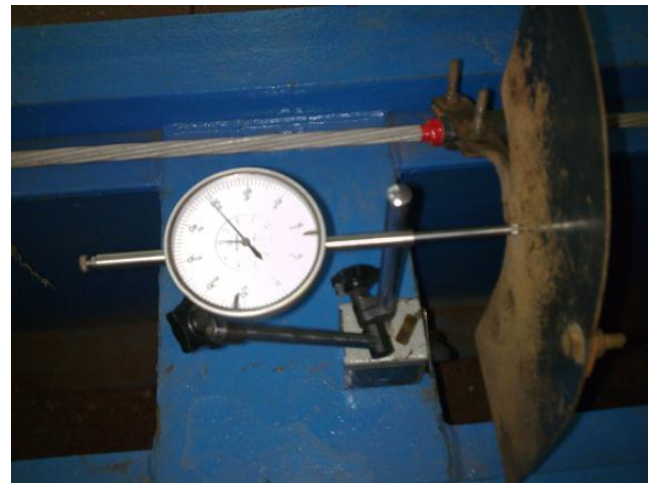
Fig. 5d Dial gauge mounting with test specimen
