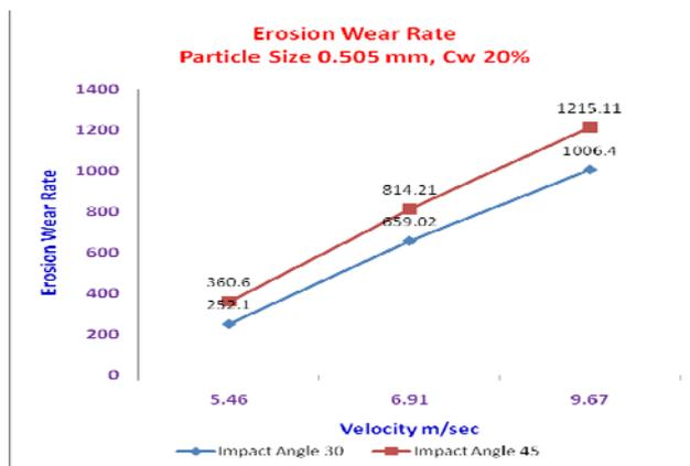
**Fig 3.4 Effect of Velocity on Erosion Wear Rate in mm/year**
