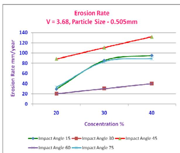
**Fig 3.3 Effect of Concentration on Erosion Wear Rate in mm/year**
