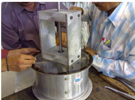
**Fig 2.1 6.6 Litre Capacity Pot Tester**
