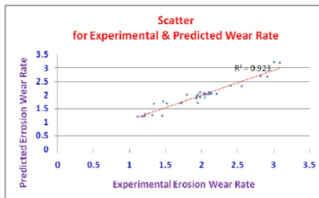
**Fig 4.1 Scatter for Experimental & Predicted Erosion Wear Rate in mm/year**
