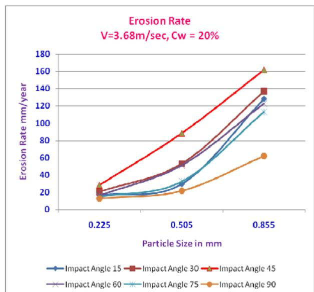
**Fig 3.2 Effect of Particle Size on Erosion Wear Rate in mm/year**
