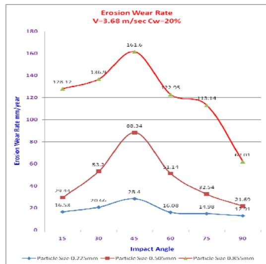
**Fig 3.1 Effect of Impact Angle on Erosion Wear Rate in mm/year**
