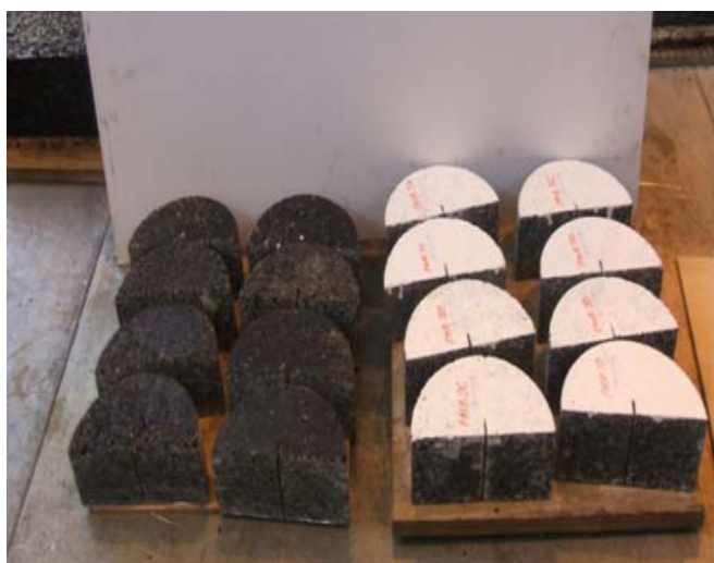
Fig. 3 Semi-circular PMB specimens
