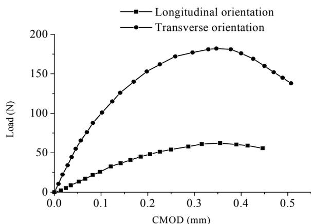
Fig.3. Load-CMOD curve for transverse and longitudinal fractured specimens obtained from the mid diaphysis of cortical tibia.
