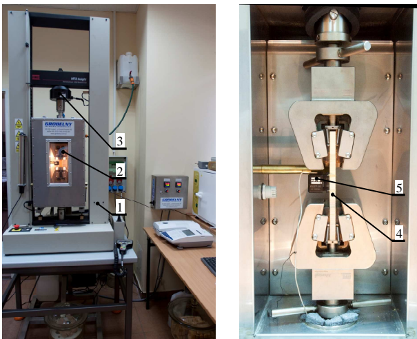
Fig. 7 MTS strength tester including climate chamber 1 – strength tester, 2 – climate chamber, 3 – load cell (measuring the applied force), 4 – specimen, 5 – mechanical extensometer
