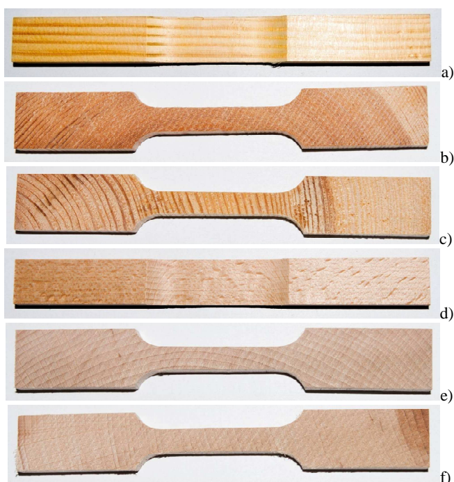
Fig. 4 Specimens: a) pine - longitudinal direction, b) pine - tangential direction, c) pine - radial direction, d) beech - longitudinal direction, e) beech - tangential direction, f) beech - radial direction
