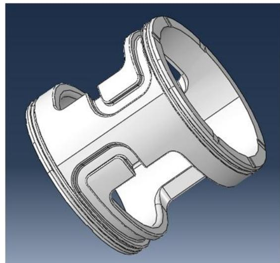
Figure 11: Isometric Model of Armature Design
