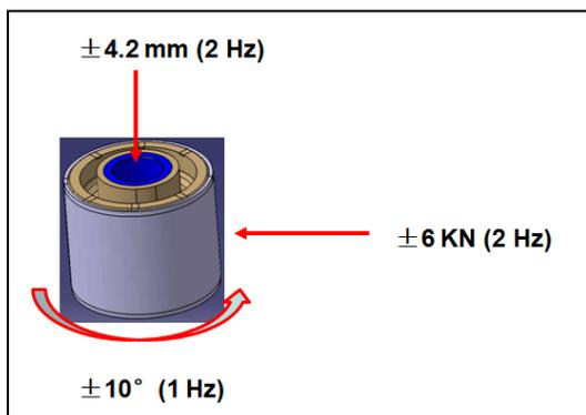
Figure 14: Durability Loading Setup
