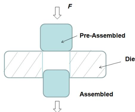
Figure 2: Out Can Swaging Process
