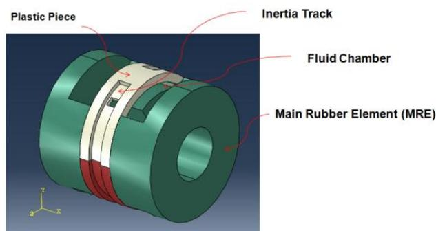
Figure 1: Typical Hydrobushing
