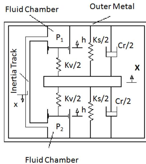
Figure 8: Hydrobushing Model
