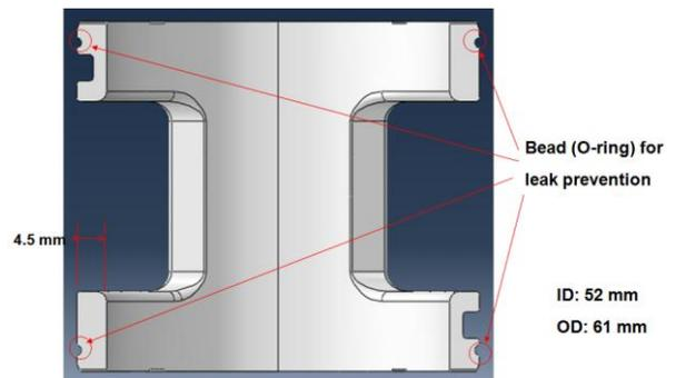
Figure 10: O-ring Groove Design
