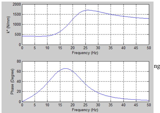
Figure 9: Predicted Dynamic Properties of Hydrobushing
