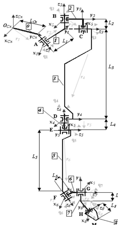
Fig. 1. The cinematic model equivalent with the human lower limb
