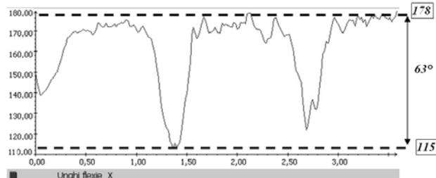
Fig. 9. The new prosthesis flexion/extension angular displacement variation, depending on time
