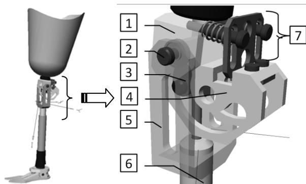
Fig. 7. Virtual model of the prosthesis used in human knee disarticulations
