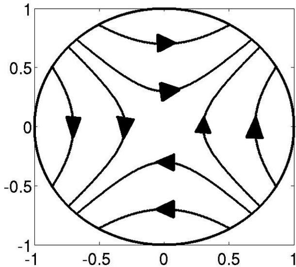
Fig. 1. Electrical current traces for the homogeneous case.
