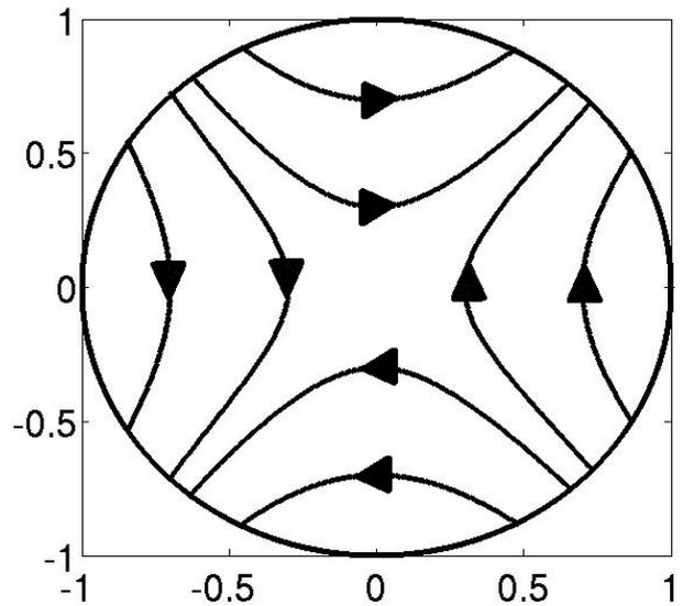
Fig. 2. Electrical current traces for the first inhomogeneous case.
