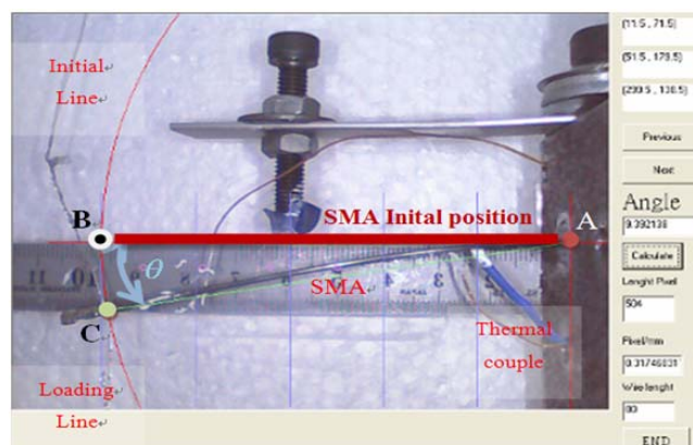
Fig. 6. A web camera's vision-capturing system used to acquire the image of the SMA-made bending actuator via a VB's dialogue.
