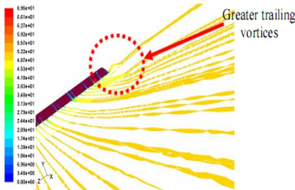
Fig. 11 Pathlines for Rectangular wing at  $\alpha = 12^\circ$
