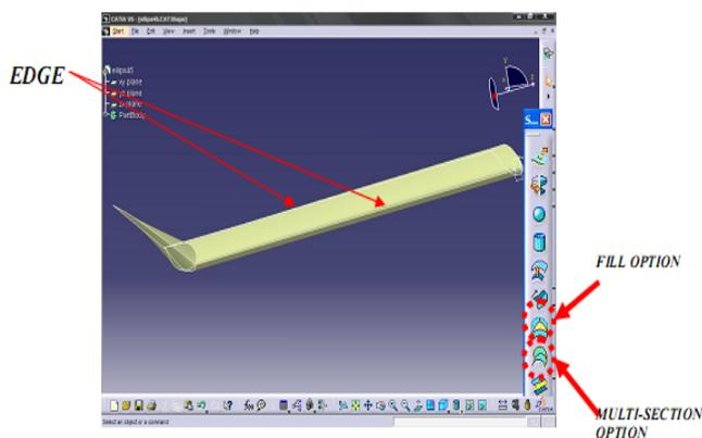
Fig. 2 Generated surface of wing and winglet
