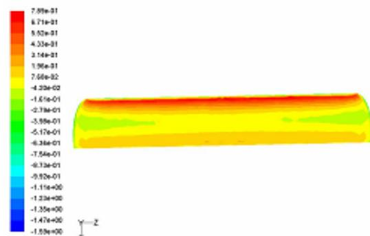
Fig. 10 Bottom  $C_p$  contours for elliptical winglet of 45 Degree Cant Angle at  $\alpha = 12^\circ$
