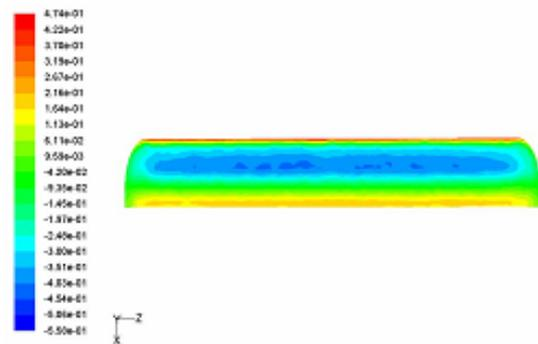
Fig. 9 Bottom  $C_p$  contours for elliptical winglet of 45 Degree Cant Angle at  $\alpha = 0^\circ$
