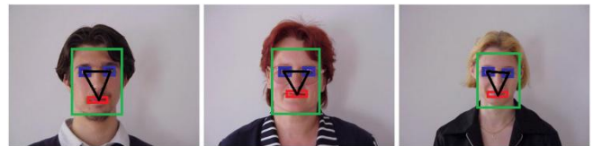
Fig. 9. Final face detection results after implementing the flexible geometric model and verification to confirm the face candidate as a face.
