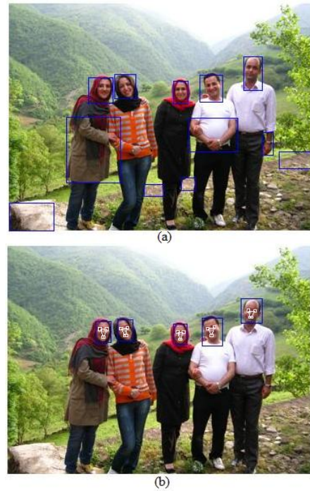
Fig. 12. A sample of detected faces in a real image with complex background. (a) face detection result using skin color segmentation, (b) face detection using skin color segmentation and component-based verification.
