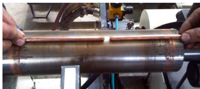
Fig. 5. Photograph of broken rotor bar parts and rotor.
