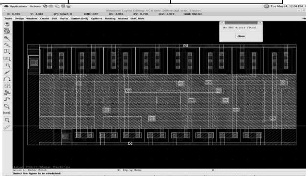
Fig12 Layout of proposed ring oscillator showing no DRC error
