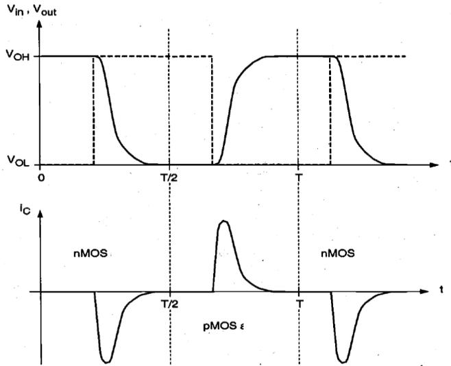
Fig.6 Input and output voltage and capacitor current waveform [2]
