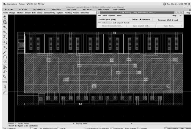
Fig13 Layout of proposed ring oscillator showing no LVS error
