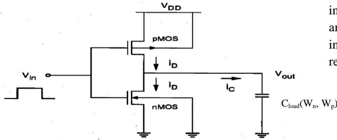
Fig.5 CMOS inverter for power analysis [2]
