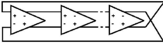
Fig.3 Basic Differential ring oscillator
