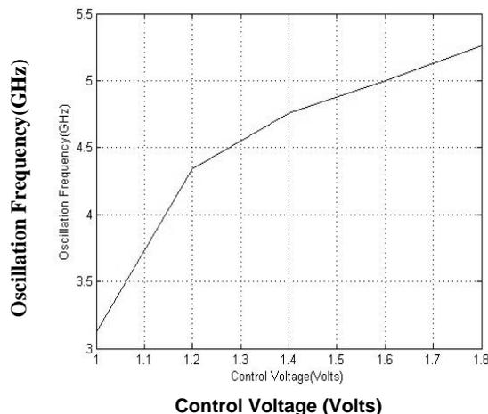
Fig.11 Frequency vs control voltage graph is shown
