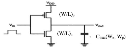
Fig.4 CMOS Inverter [2]
