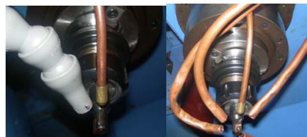
(a) One nozzle+MQL (b) Four nozzles+MQL
