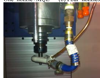
(c) Combined cold air and MQL nozzle
