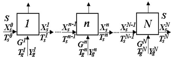
Fig. 1. Scheme of the multistage fluidized drying process.
