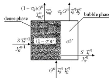
Fig. 2. Scheme of two-phase fluidized bed.
