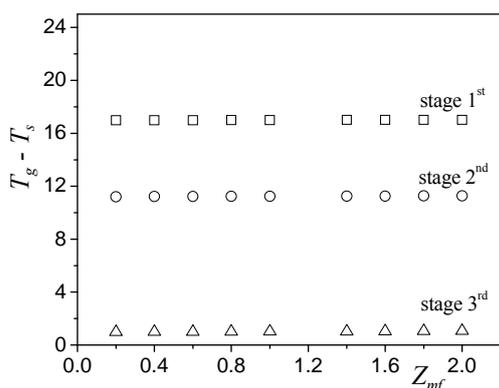
Fig. 5. Optimal substituted driving forces for heat convective transfer on stages 1<sup>st</sup>, 2<sup>nd</sup>, and 3<sup>rd</sup>.
