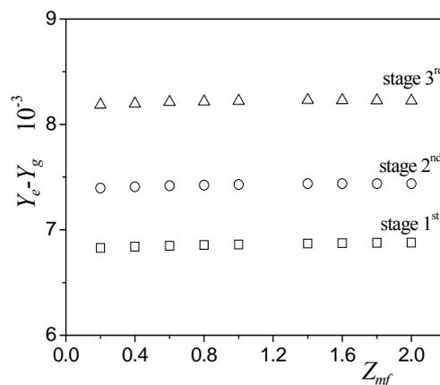
Fig. 6. Optimal driving forces for mass transfer on stages 1<sup>st</sup>, 2<sup>nd</sup>, and 3<sup>rd</sup>.
