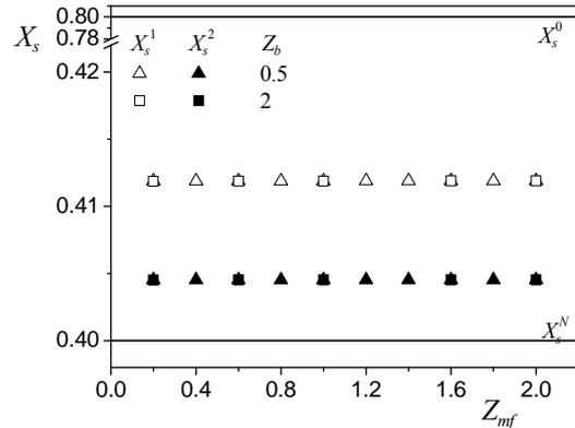
Fig. 3. Solid moisture content after first  $X_s^1$  and second stage  $X_s^2$  as a function of coefficient  $Z_{mf}$  and for two values of coefficient  $Z_b$ .
