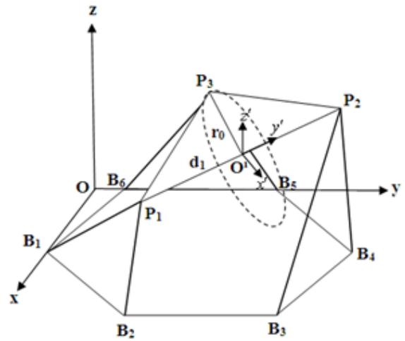
Fig. 8. The vertex  $P_3$  moving in the circle with radius  $r_0$ .
