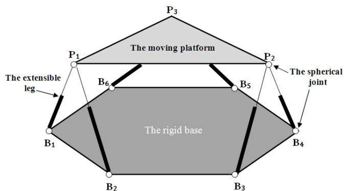
Fig. 1. 6-3 Stewart Platform Mechanism.
