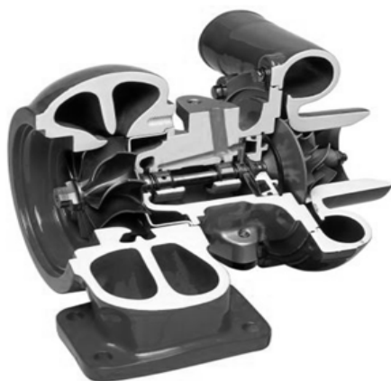
Fig. 1. Turbocharger cut-away highlighting the twin-entry volute geometry, allowing differently pulsed exhaust gases to remain separate.
