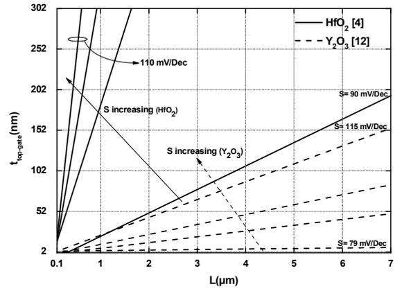
Figure 4. Graphical abacus which allows studying the scaling capability of the G-FETs
