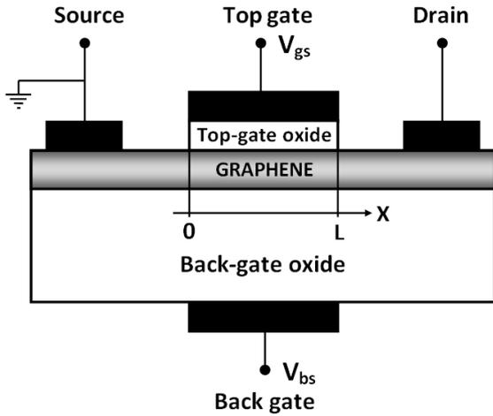
Figure 1. 2D Cross section Dual-Gate G-FET considered in this work: Graphene channel and metal-like source/drain regions are used in this study
