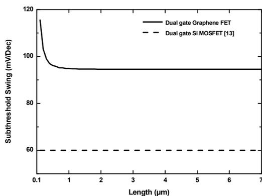
Figure 3. Subthreshold swing versus channel length
