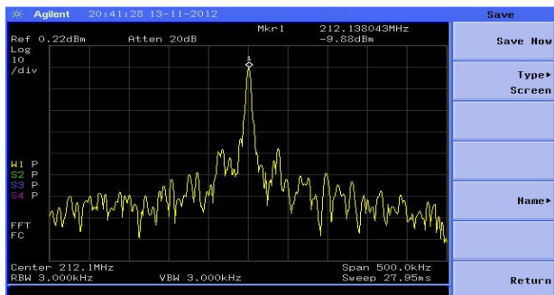
Fig.4: Output spectrum of the frequency synthesizer at 212.1 MHz
