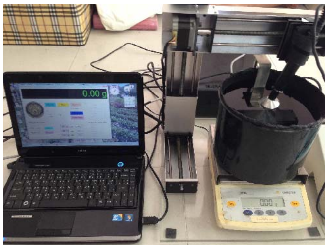
Fig. 2. Photograph of the developed ultrasound power meter with the three axis positioning system
