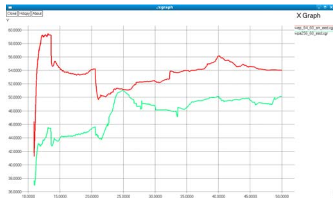
Fig. 7. Comparison of variation in End to End Delay for WEP and WPA for wireless LAN comprising of 60 nodes
