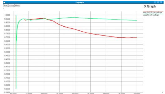
Fig. 1. Comparison of variation in PDF for WEP and WPA for wireless LAN comprising of 20 nodes
