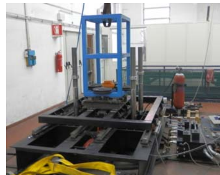
Fig. 13. Cabinet on the shake-table.
