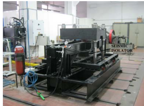
Fig. 2. The earthquake simulator in the seismic isolator configuration
