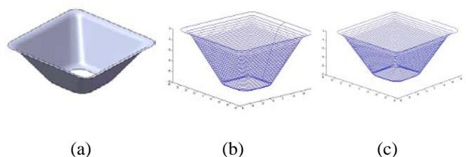
Fig 5: (a) CAD Model (b) Contour Tool path (c) Helical Tool path
