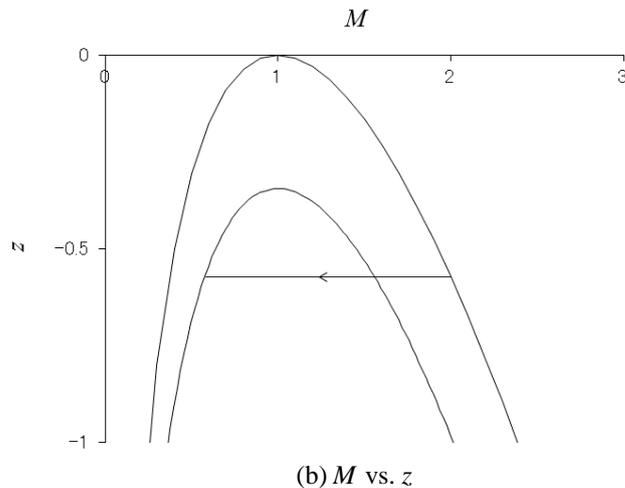
Fig.3 Open channel flow over a hump ( $z$  in the figure for  $\frac{z-z_*}{y_*}$ )
