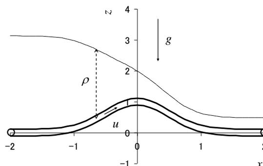
(b) One-dimensional compressible flow under gravity
