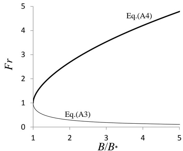
Fig. A1 Hydraulic Laval nozzle - Horizontal open-channel flow with varying width
