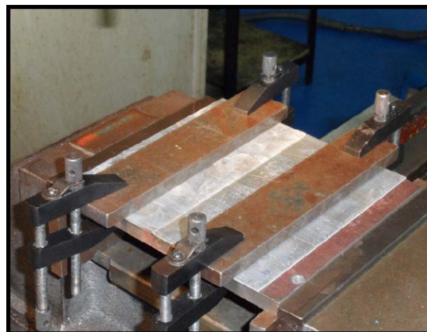
Fig. 2. Welding fixture for FSW.
