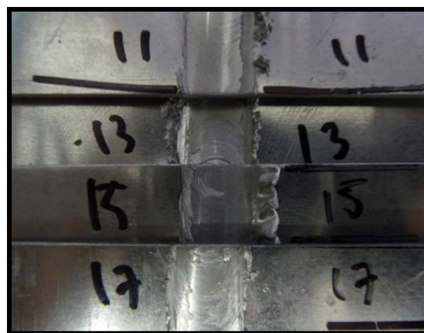
Fig.6. Welded sample used for roughness.
