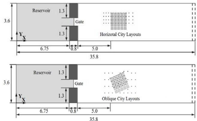
Fig. 1 Set-up of the experiment by Soares-Frazão and Zech (2008) [6]
