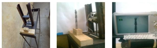
**Figure 3 Setup for capturing the images of drill tool**
