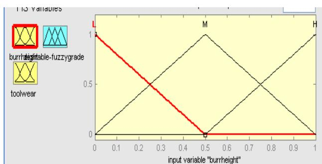
Fig.8 Membership functions of burr height and tool wear
