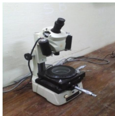
**Figure 2 Tool makers microscope**
